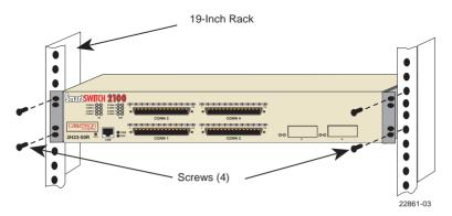
Figure 3-4 Installing the Device in a Rack
